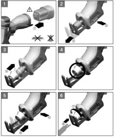
WARNING: ALWAYS remove battery pack before cleaning or maintenance.
